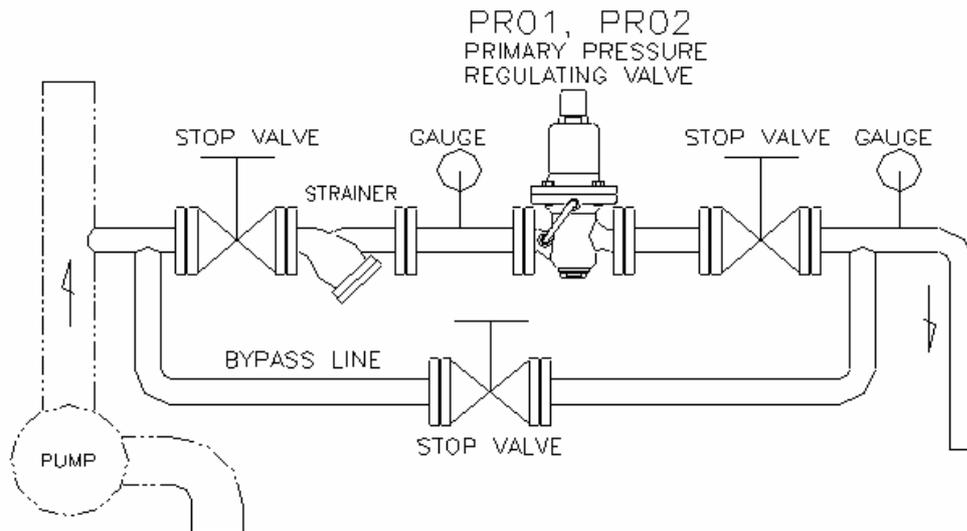
4.2 Please install stop valves, a strainer and a bypass line as exemplated above.
