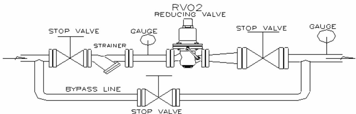
4.2 As shown in the piping example, install straight pipe part before and after the pressure reducing valve, and install stop valves, strainer, safety valve, pressure gauges and a bypass line.
