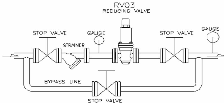
4.2 As shown in the piping example, install straight pipe part before and after the pressure reducing valve and also install stop valves, strainer, safety valve, pressure gauges and a bypass line.
