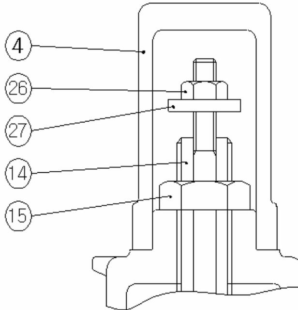
Take off cap(4), loosen lock nut(15) and turn down the adjusting screw(14) to the right(clockwise viewing from above) to raise set pressure and turn up the left (anti-clockwise viewing from above) to lower the set pressure.
